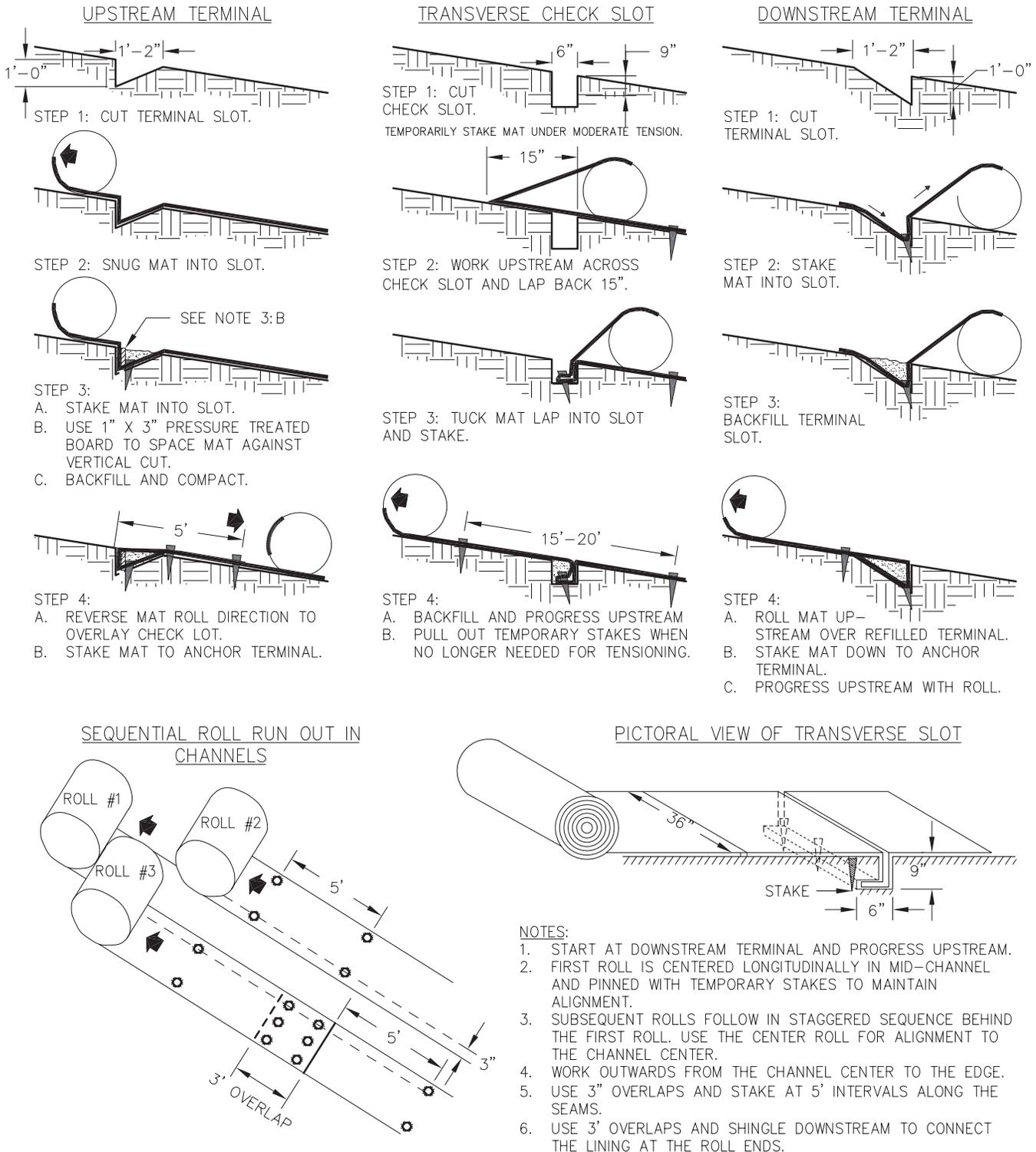
Figure 6-10.1 - Typical Installation Guidelines for Matting and Blankets
