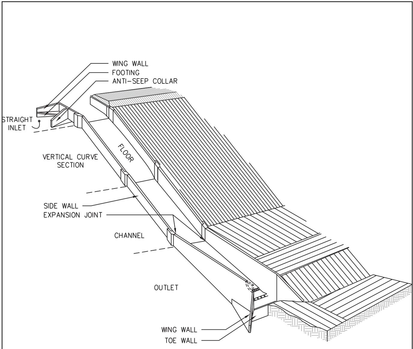
**Figure 6-22.7 Chute Spillway**
