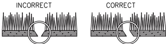
BUTTING: ANGLED ENDS CAUSED BY THE AUTOMATIC SOD CUTTER MUST BE MATCHED CORRECTLY.
