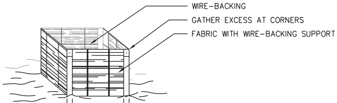
**Figure 6-28.1 - Fabric and Supporting Frame For Inlet Projection**
