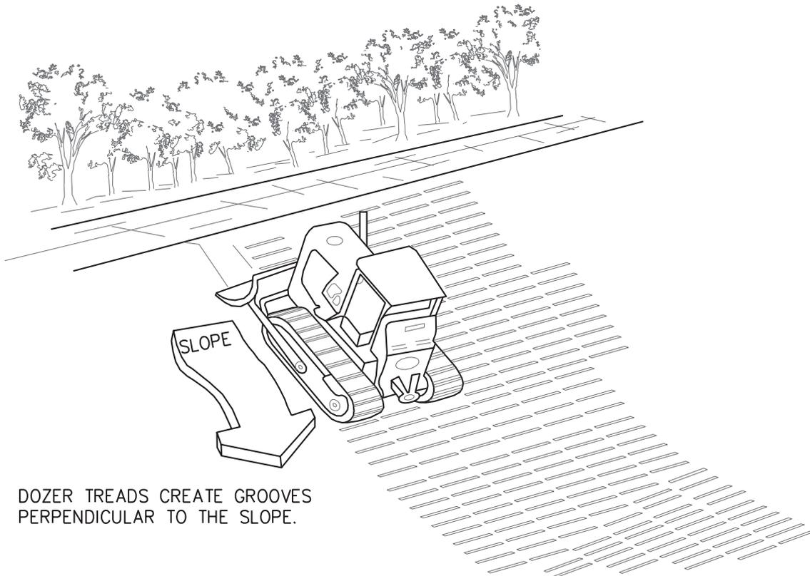
DOZER TREADS CREATE GROOVES PERPENDICULAR TO THE SLOPE.
