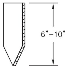
IN CRITICAL AREAS, SECURE SOD WITH NETTING USING STAPLES.
