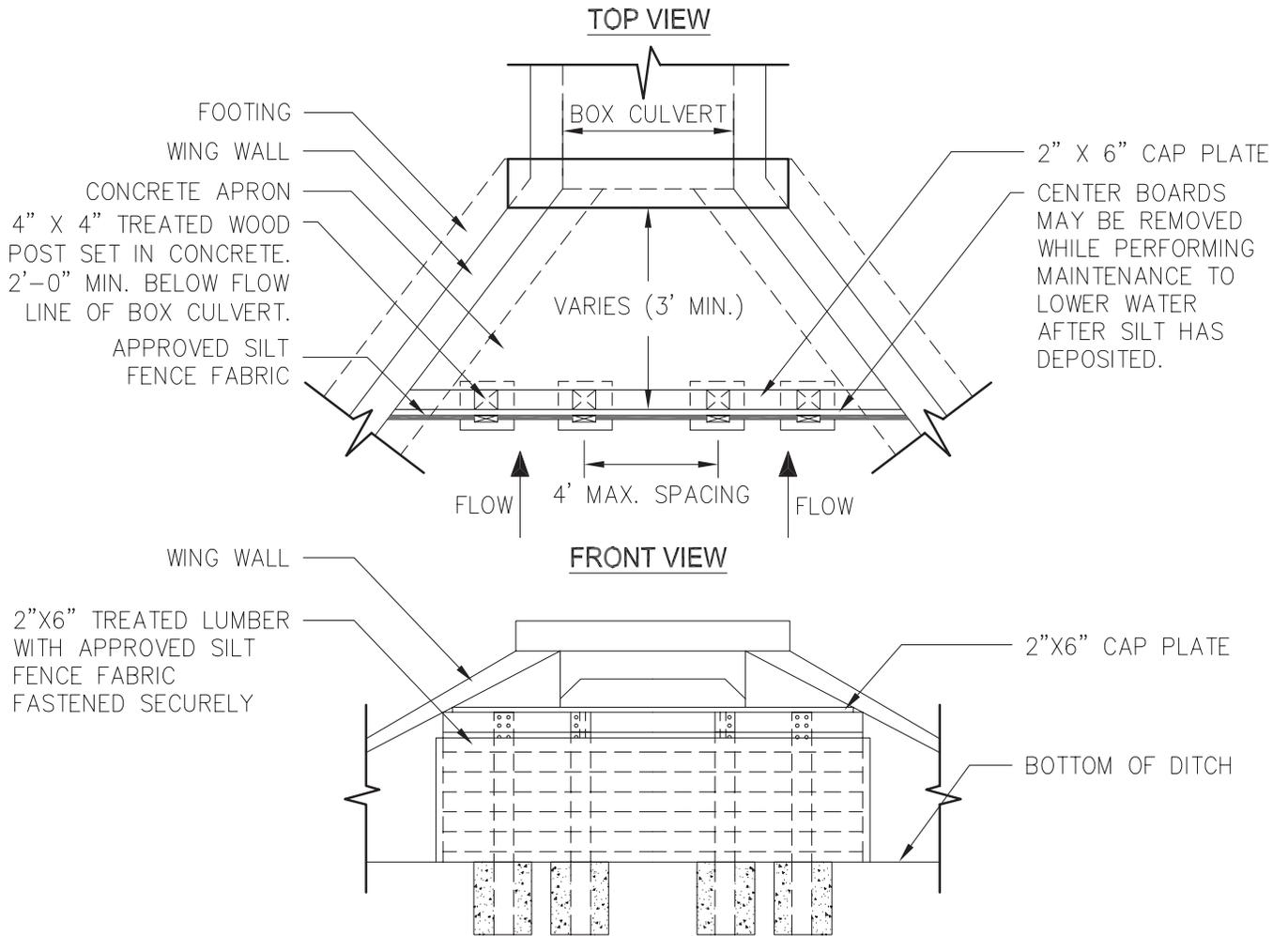
**Figure 6-26.4 Silt Control Gate**
