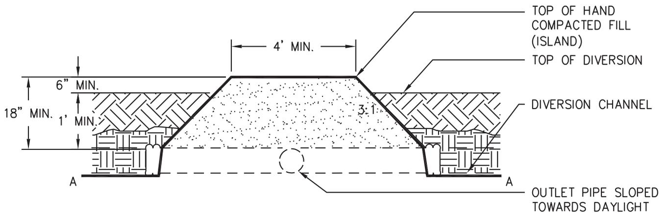
MAKE ALL PIPE CONNECTIONS WATERTIGHT AND SECURE SO THAT THE JOINTS WILL NOT SEPARATE IN USE.
