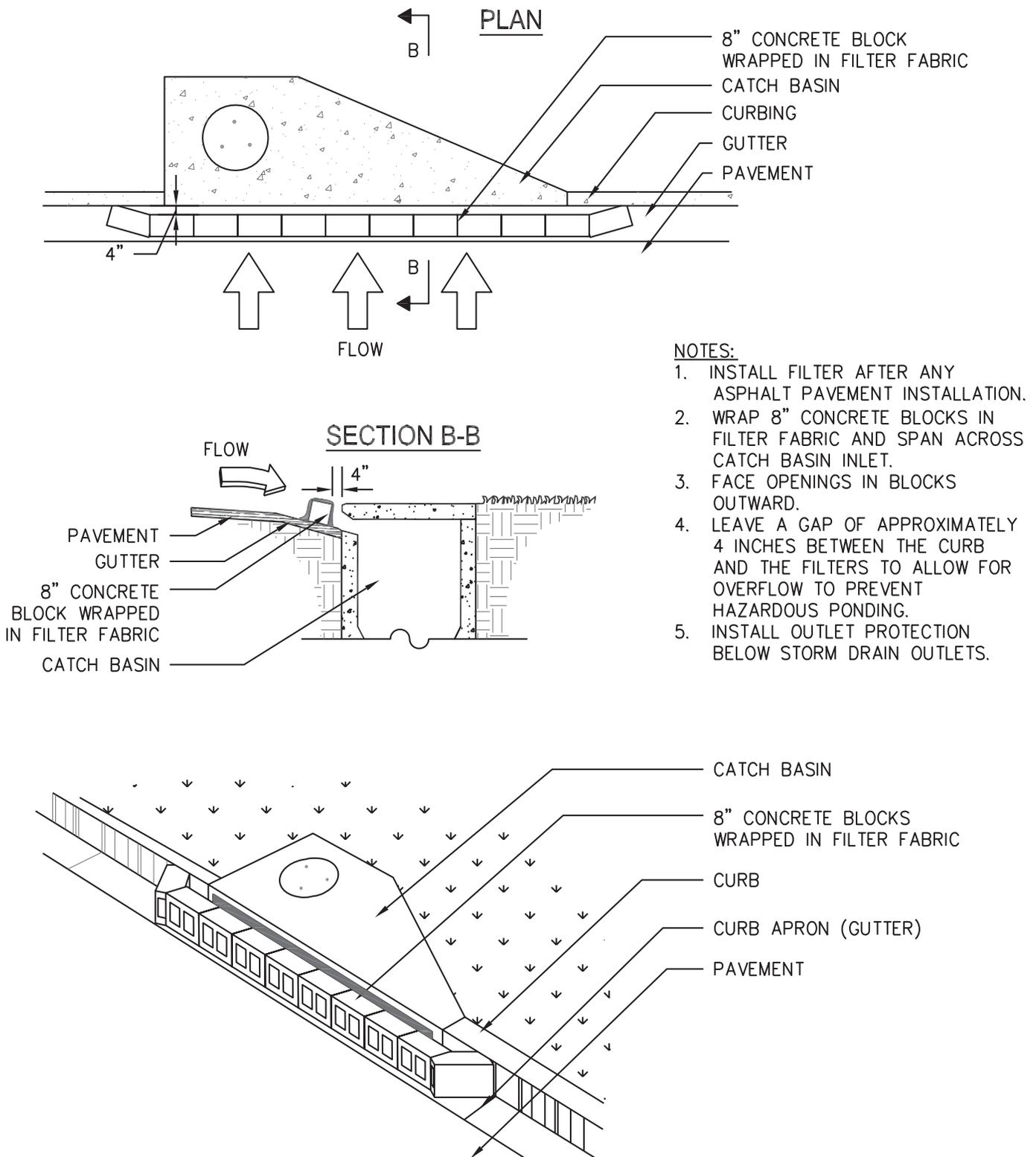
Figure 6-28.6 Curb Inlet Filter "Pigs in Blanket"
