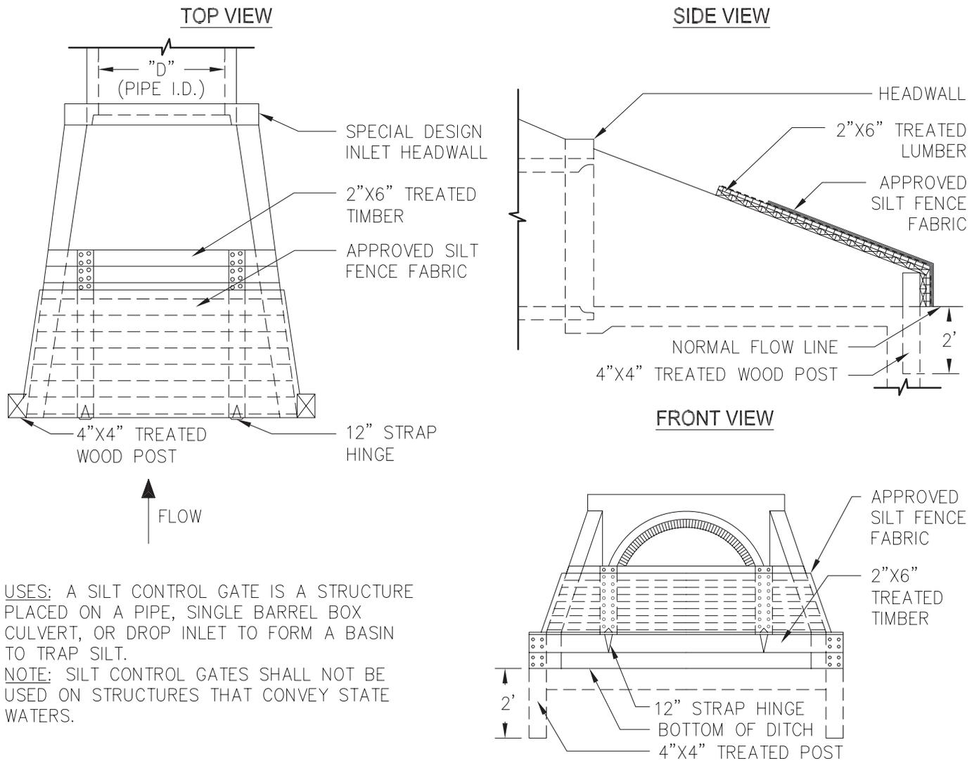
USES: A SILT CONTROL GATE IS A STRUCTURE PLACED ON A PIPE, SINGLE BARREL BOX CULVERT, OR DROP INLET TO FORM A BASIN TO TRAP SILT.
