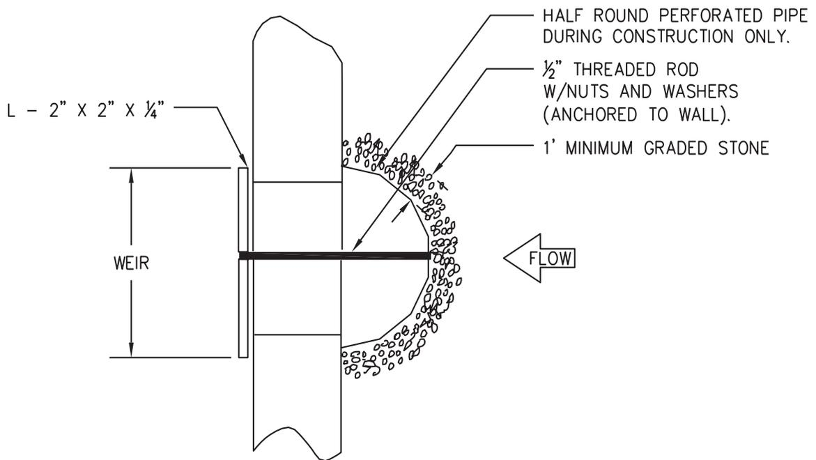
Figure 6-26.1 Perforated Half- Round Pipe with Stone Filter
