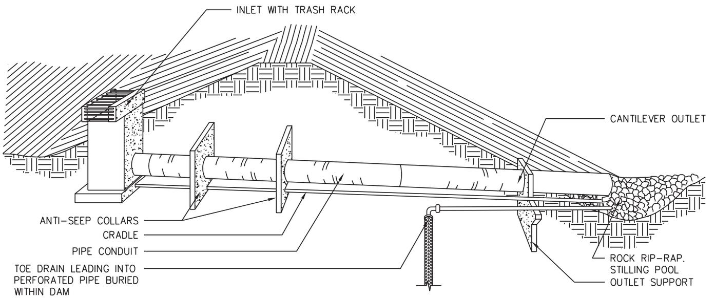
**Figure 6-22.5 Drop Inlet Spillway**
