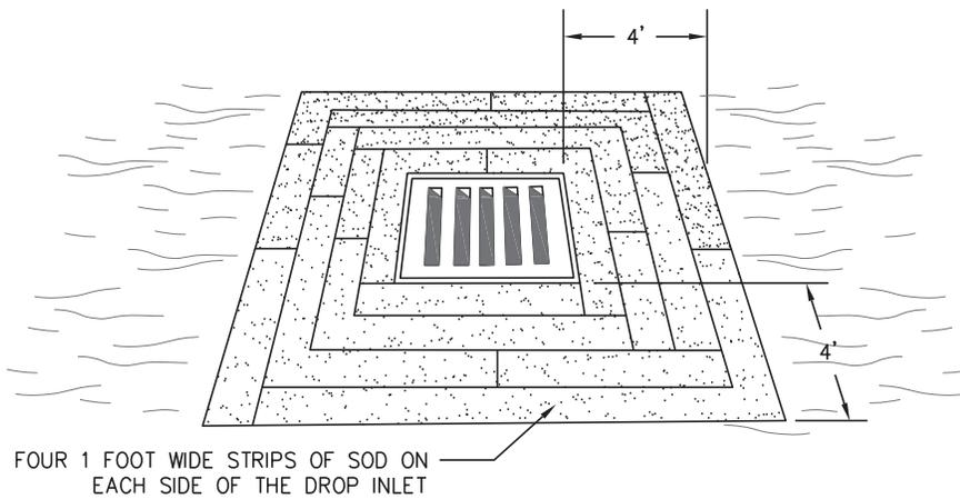
Figure 6-28.5 Sod Inlet Protection
