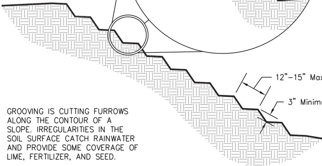
GROOVING IS CUTTING FURROWS ALONG THE CONTOUR OF A SLOPE. IRREGULARITIES IN THE SOIL SURFACE CATCH RAINWATER AND PROVIDE SOME COVERAGE OF LIME, FERTILIZER, AND SEED.
