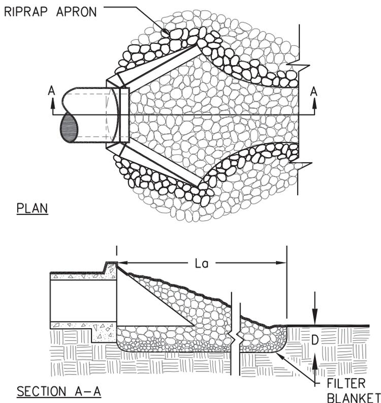
Figure 6-34.3 - Riprap Outlet Protection (Modified From Va SWCC)
